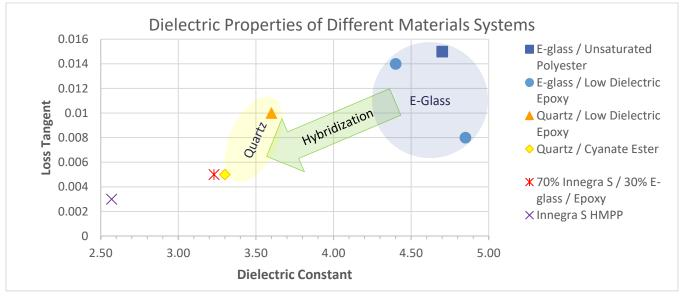
Innegra S hybrid FRP composites have previously been shown to have higher impact resistance and damage tolerance than composites made from brittle reinforcement fibers alone. Hybridization of a FRP composite with Innegra S fibers can therefore allow designers to create a composite radome structure that is better able to satisfy the full range of requirements.
